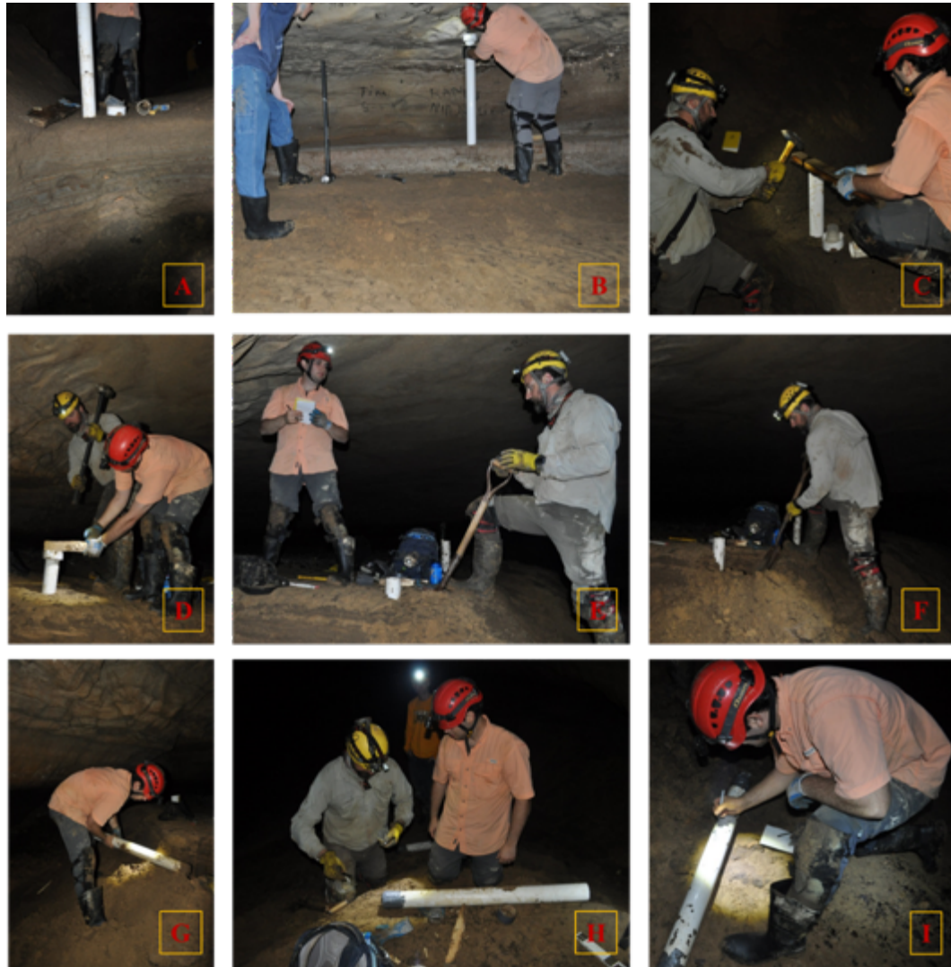
Figure 22. The extraction process of collecting sediment cores. A) Equipment used for core extraction. B) Extraction location limited to cave roof. C) Manual hammering PVC core barrel into sediment using a small hammer. D) Manual hammering PVC core barrel into sediment using a sledgehammer. E) PVC core barrel located in sediment bank after manual hammering. F) Manual digging of PVC core to reduce sediment disturbance. G) Retrieval of PVC core from sediment bank. H) PVC cores packed and sealed to avoid disturbance during transport. I) The core is marked in detail, referencing survey station markers, core name, and stratigraphic up.
