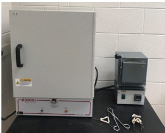
Figure 23. LOI conducted using a conventional oven (Left) and muffle furnace (Right).
