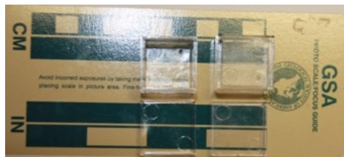
Figure 24. Specially designed 2 \text{ cm}^3 plastic cubes. (Photo by Brooks Ellwood)
