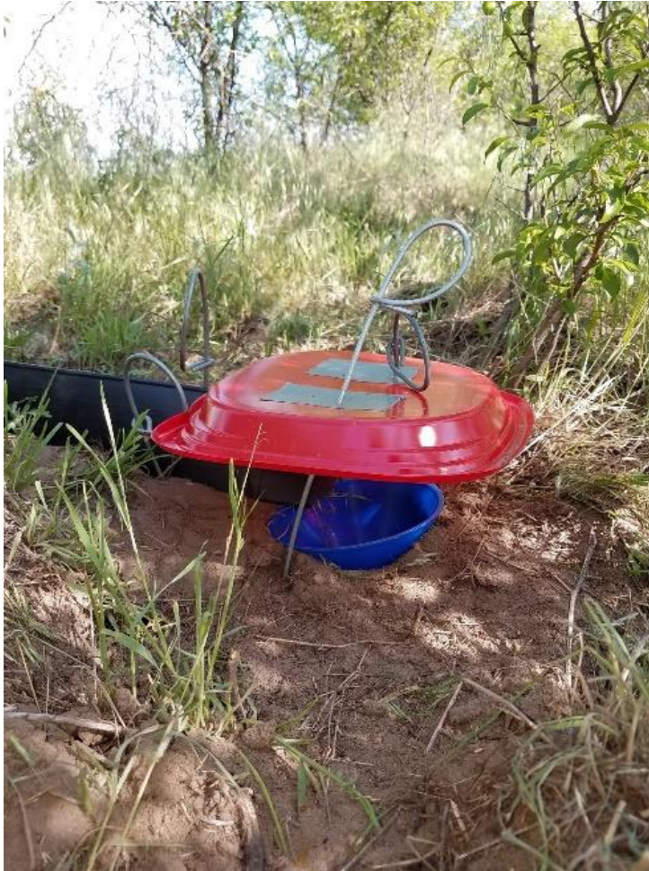
Figure 1. Closeup view of a pitfall trap for carabid trapping. Pitfall trap arrays consisted of two traps separated by 300 cm of plastic drift fence. Sampling occurred in a grassland characterized by prairie sand dunes. Each trap consisted of a plastic cup dug in the ground. A second cup was placed within and was removed to empty traps. A cattle ear tag impregnated with permethrin was used as a killing agent. Each trap was equipped with a funnel to increase capture rates of invertebrates and decrease vertebrate bycatch. An inverted plastic plate was used as a rain guard to prevent flooding of traps.
