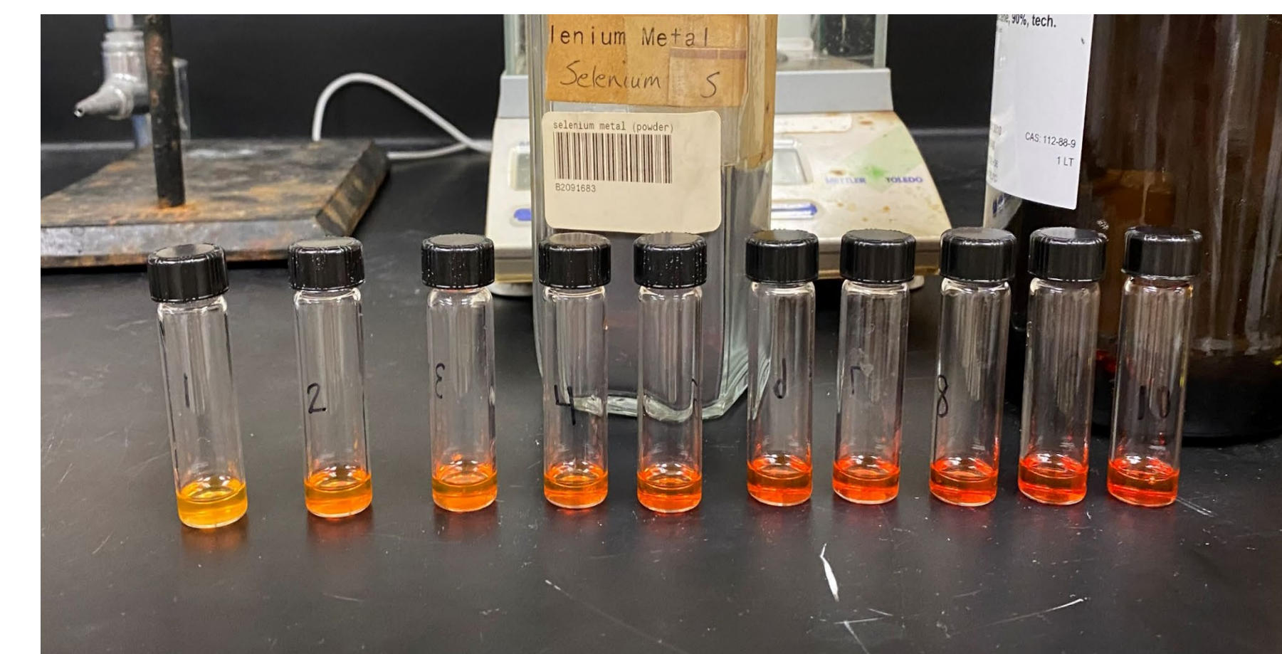
Figure 4. Synthesized CdSe Quantum Dots passivated with trioctylphosphine, TOP
