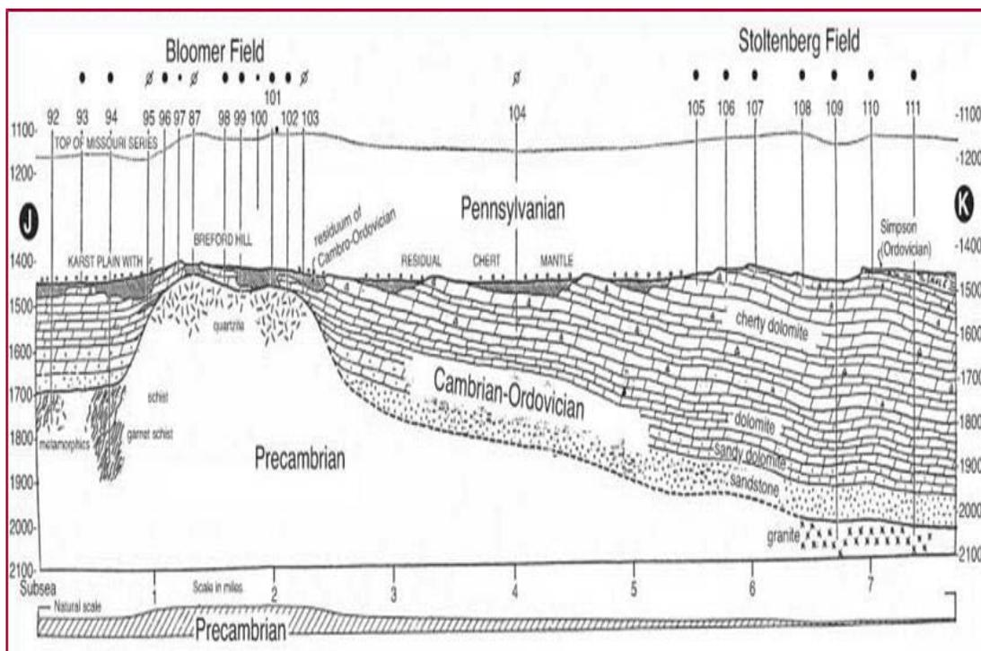
**Figure 12:** Cross section showing differential erosion of the Precambrian basement rocks, relationship of the overlying Cambrian-Ordovician strata, and karstic features paleo-highs associated with the upper Arbuckle unconformity surface (obtained from Walters, 1958 and modified).
