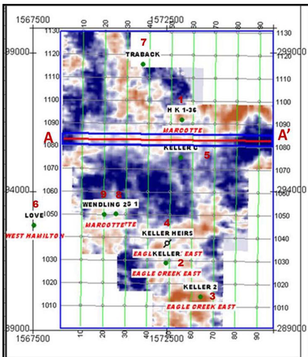
**Figure 49:** Seismic amplitude map (time slide) on top of the Arbuckle Group. High amplitudes are shown in brown/light grey, and low amplitudes are shown in blue/dark color.
