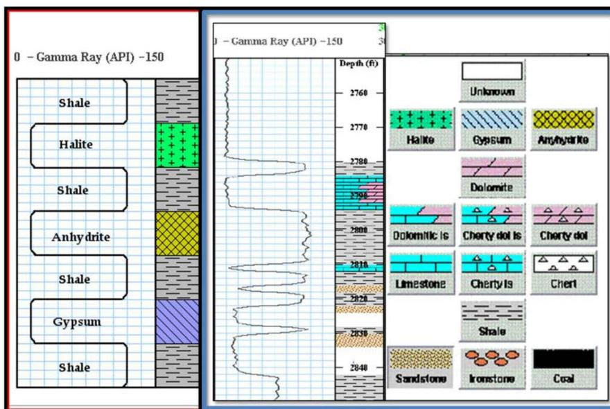
**Figure 22:** Gamma-ray (API) curve responses to different lithologies (Obtained from KGS and modified).
