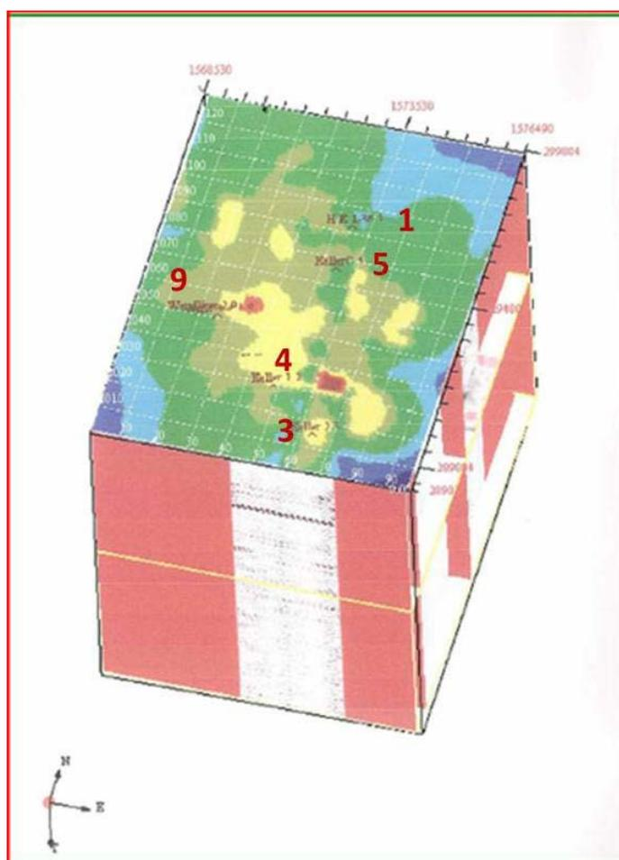
**Figure 52:** 3-D Seismic data volume cube from the Keller seismic survey.
