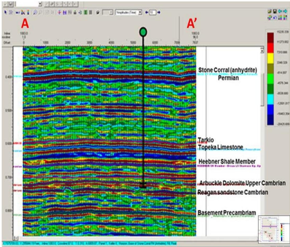
**Figure 47:** The Keller 3-D seismic profile (amplitude time) was interpreted and geologically calibrated (tied) with the local well data (green circle and black line). Seismic reflectors are correlated (tied) to the stratigraphic tops.
