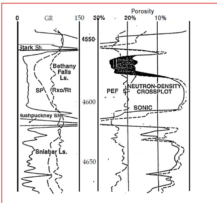
**Figure 23:** Combined logs showing the averaged neutron-density porosity log along with a sonic log in a Pennsylvanian limestone-shale sequence in a Kansas well (Obtained from KGS and modified).
