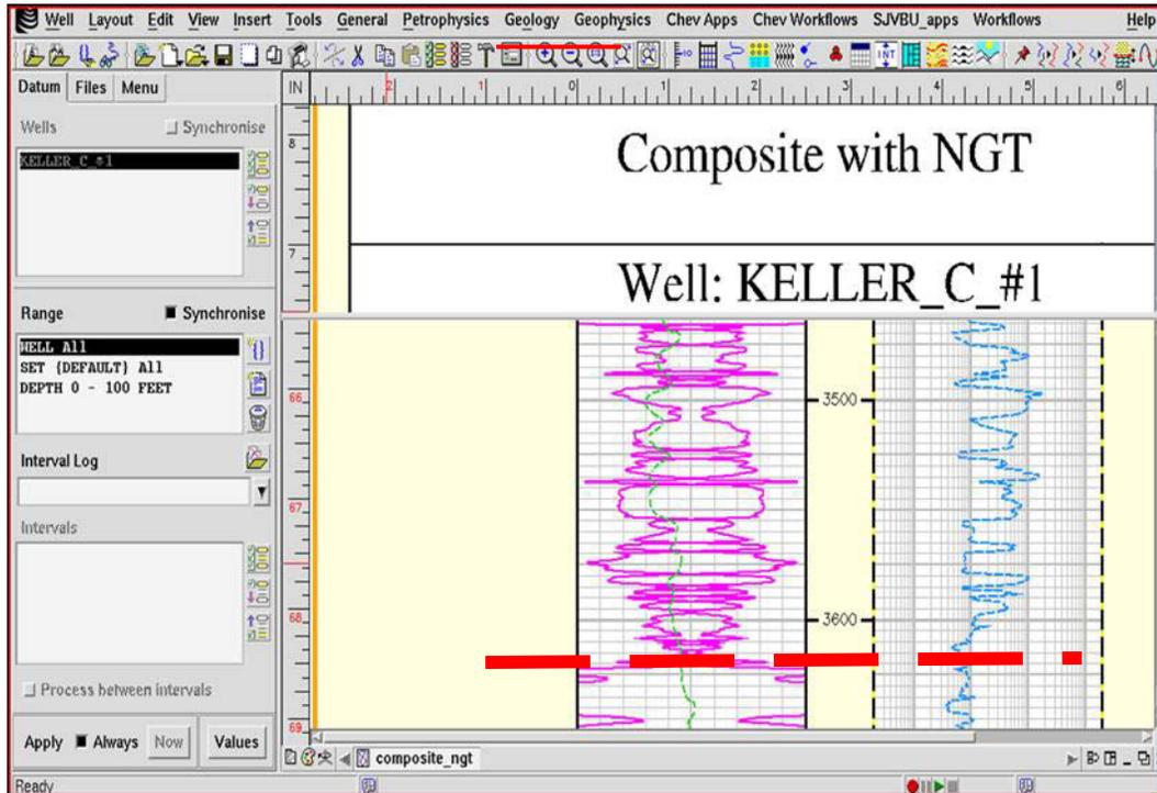
**Figure 32:** Composite log of well Keller\_C\_#1 (Well #5) with two gamma-ray (GR) curves, plotted in inverted scales, to visualize changes in lithology and a resistivity curve (compressed) showing the top of the Arbuckle.
