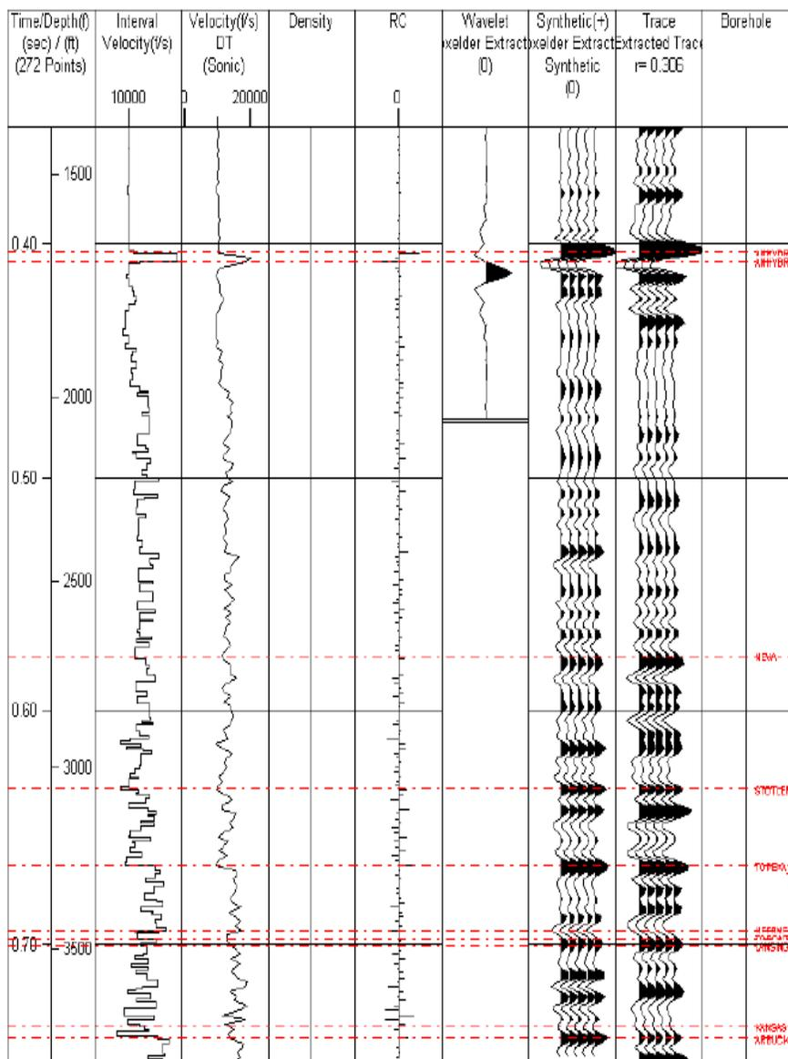
**Figure 44:** Synthetic seismogram created from sonic and density logs and used to tie and calibrate known stratigraphic tops to a seismic trace of a 3-D seismic survey recorded near the research area (Obtained from Nissen et al., 2004 and modified).
