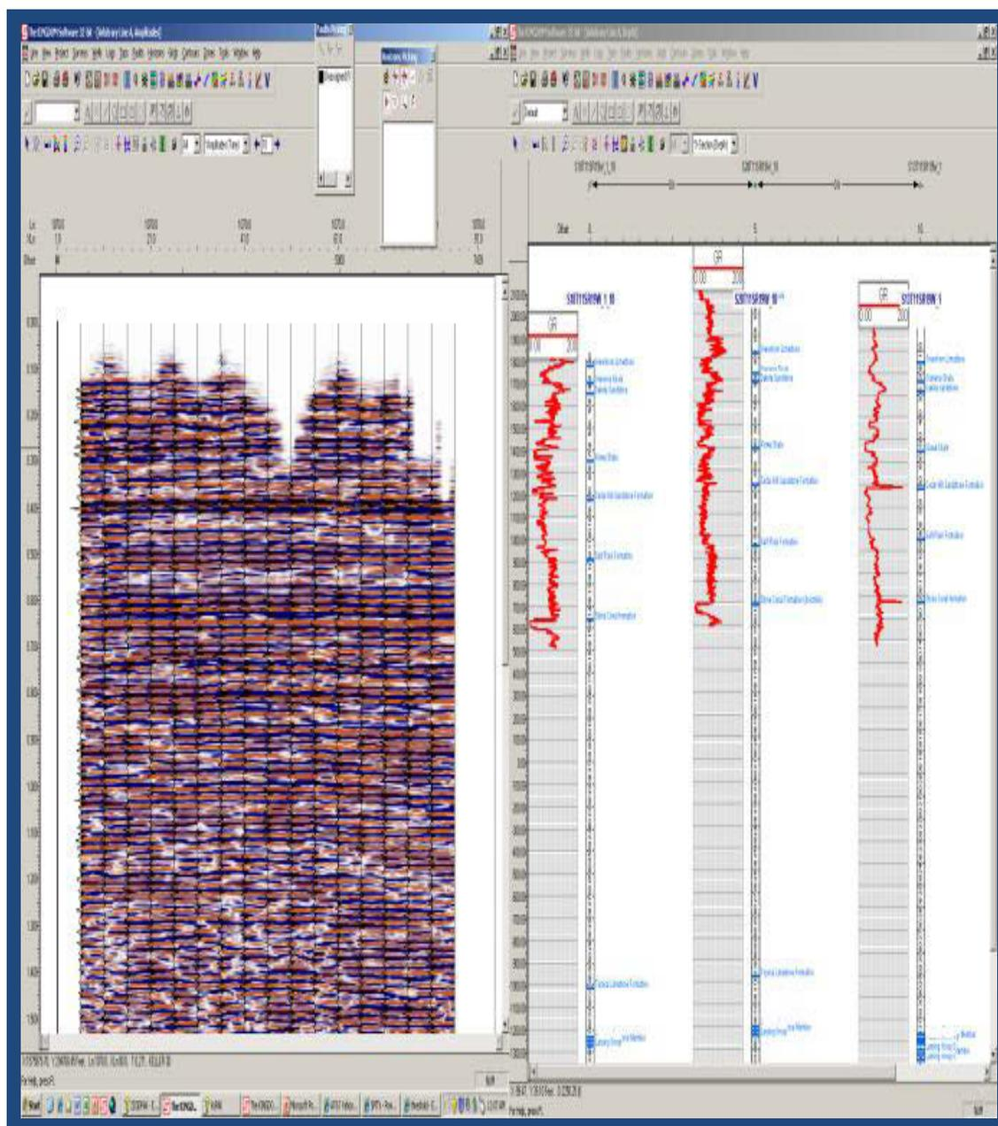
**Figure 46:** A carefully calibrated and interpreted seismic cross section identifying the tops of the stratigraphic horizons, from the Keller 3-D seismic survey.
