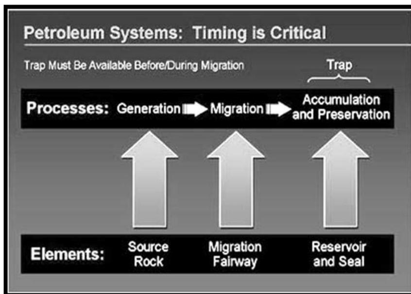
**Figure 15:** Elements and processes of the Petroleum System (Obtained from Geochemical International Solutions <http://www.geochemsol.com/analitical-basinmodeling.html>)
