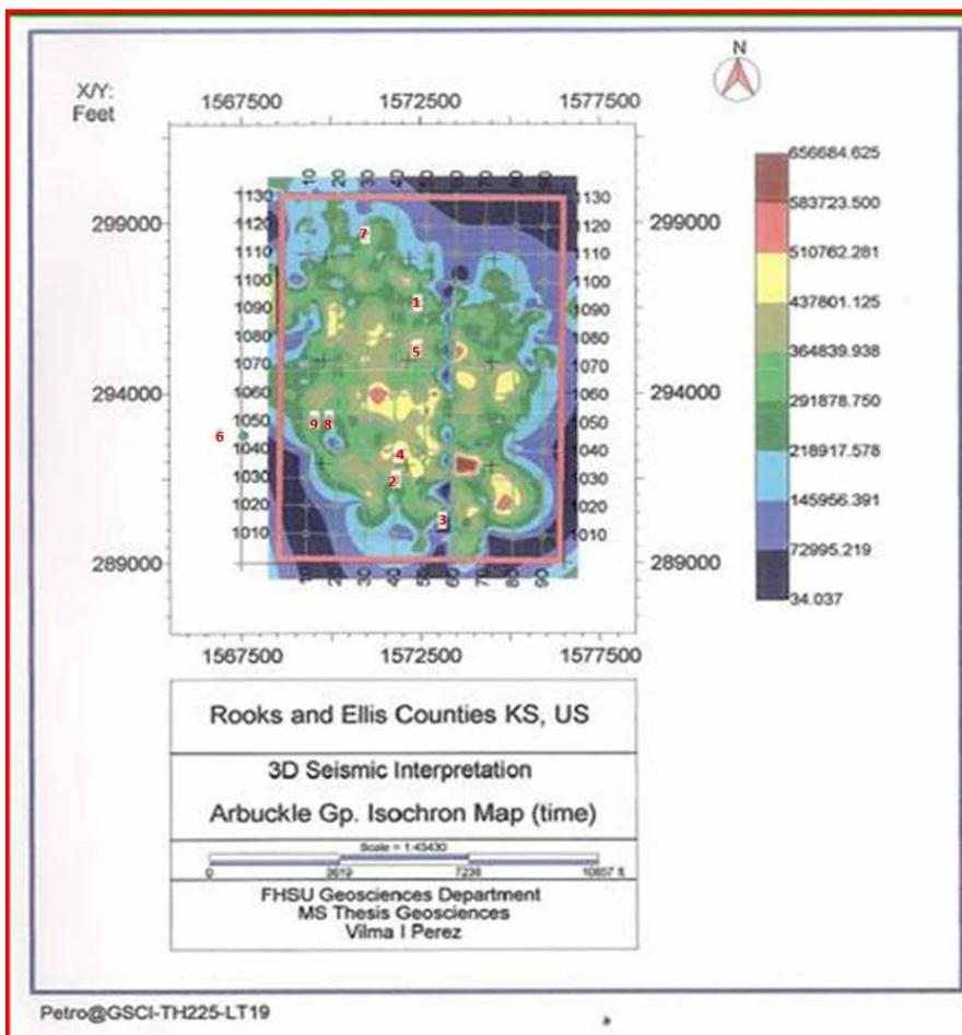
**Figure 50:** Isochron map (seismic time) of the study area. A thickness map: from the top of the Arbuckle Group to the top of the Precambrian basement. Map was created using Seismic Micro Tecnology (SMT) Kingdom Suite software (version 8.2, 2011).
