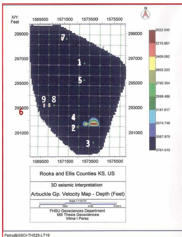
**Figure 51:** Attribute Map (Velocity) on top of the Arbuckle Group with eight oil producing wells (1-3 and 5-9) and one dry well (4). Map was created using Seismic Micro Technology (SMT) Kingdom Suite software.
