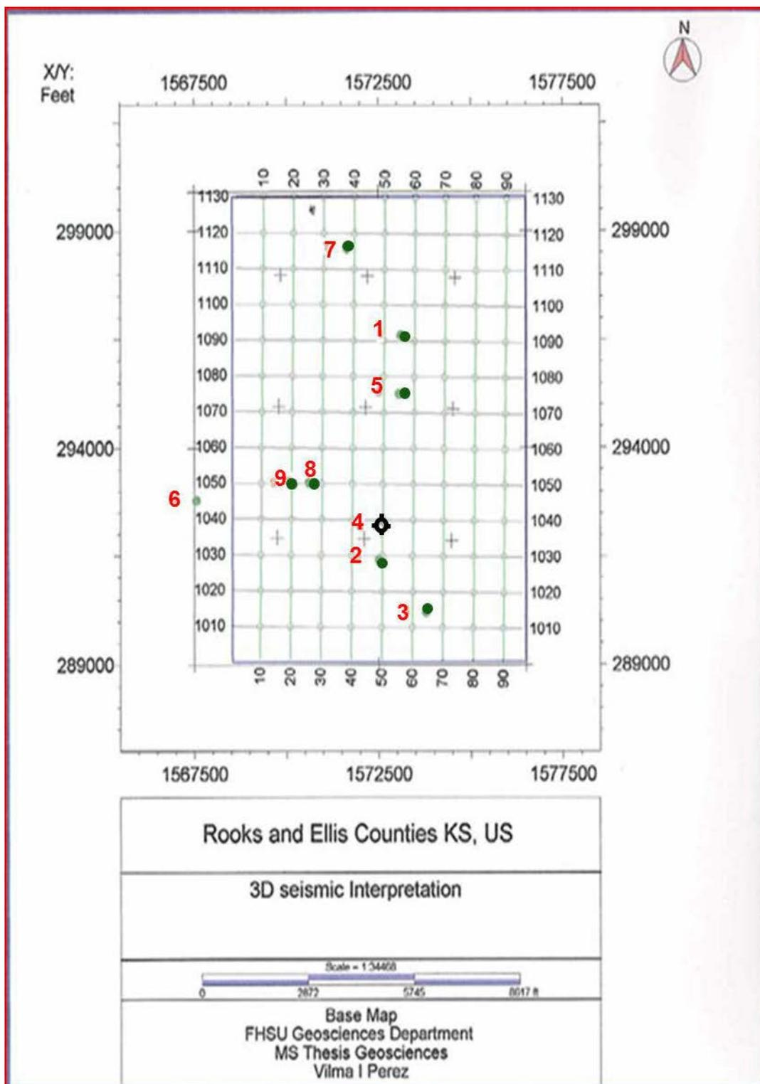
**Figure 41:** Base map showing the extent of the 3D seismic data (research area) and location of the 8 productive oil wells (solid dots ) and a dry well (#4, black dot ).
