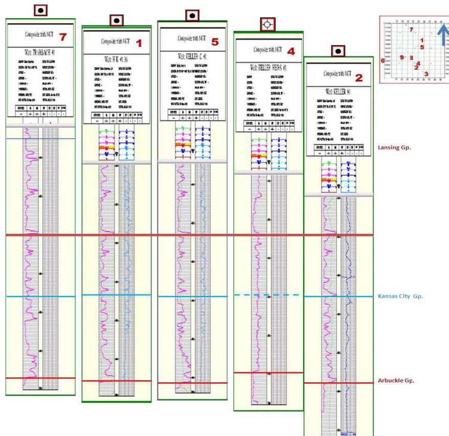
**Figure 31:** N-S Stratigraphic correlation of wells (7,1,5,4,and 2) located within the research area. Gamma-ray curve abruptly shifts to the left (low values) when the Arbuckle is logged.
