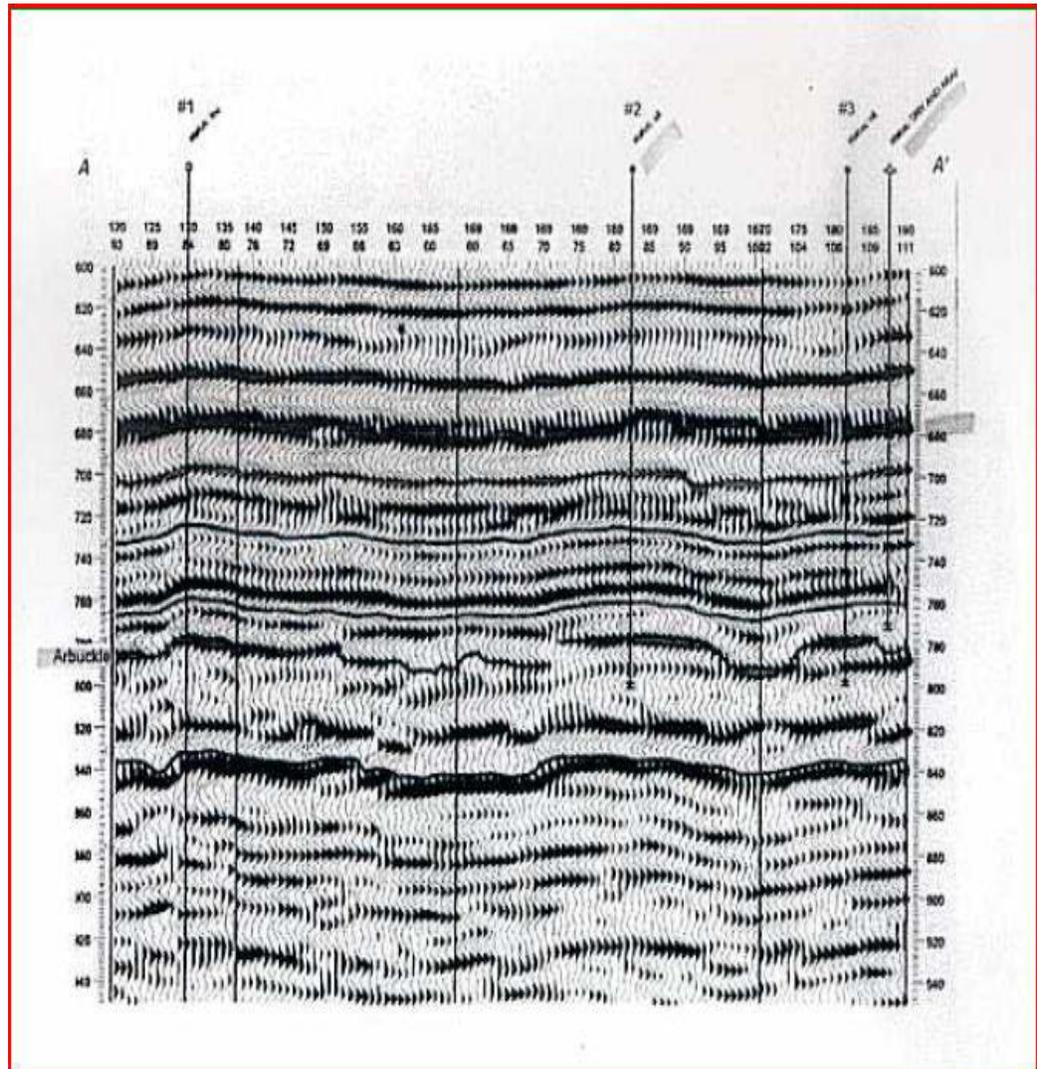
**Figure 45:** Seismic profile from a 3-D seismic survey recorded near the research area and calibrated with the well data. (Obtained from Nissen et al., 2004 and modified).
