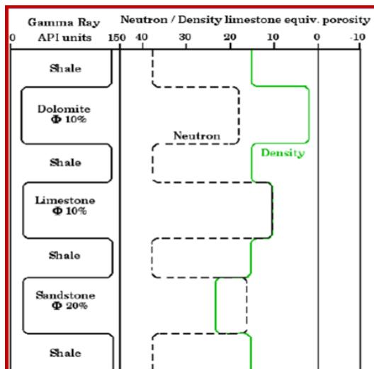
**Figure 30:** Readings of the gamma-ray (GR), the Density, and the Neutron logs in carbonates (Obtained from KGS and modified).
