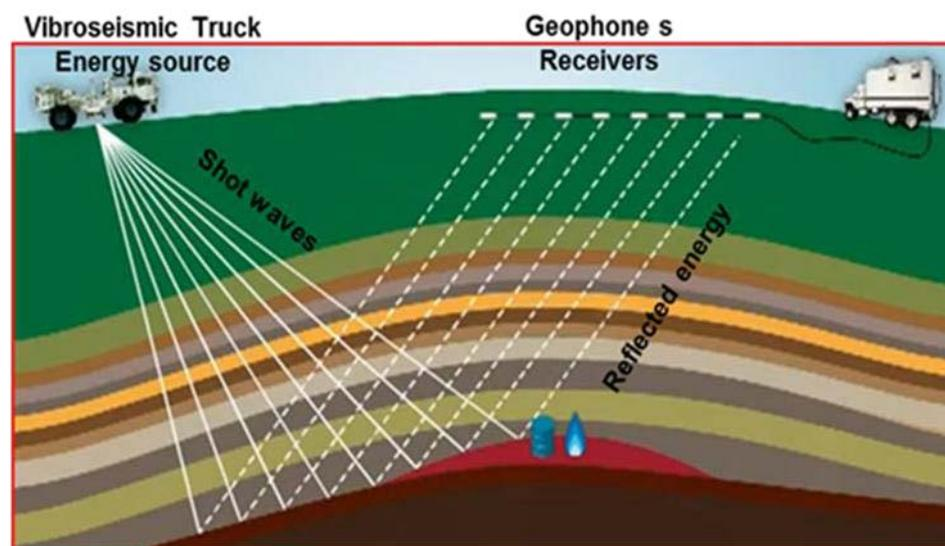
**Figure 39:** Acquisition of 3-D seismic data (Obtained from Schlumberger Oil Glossary and modified)
