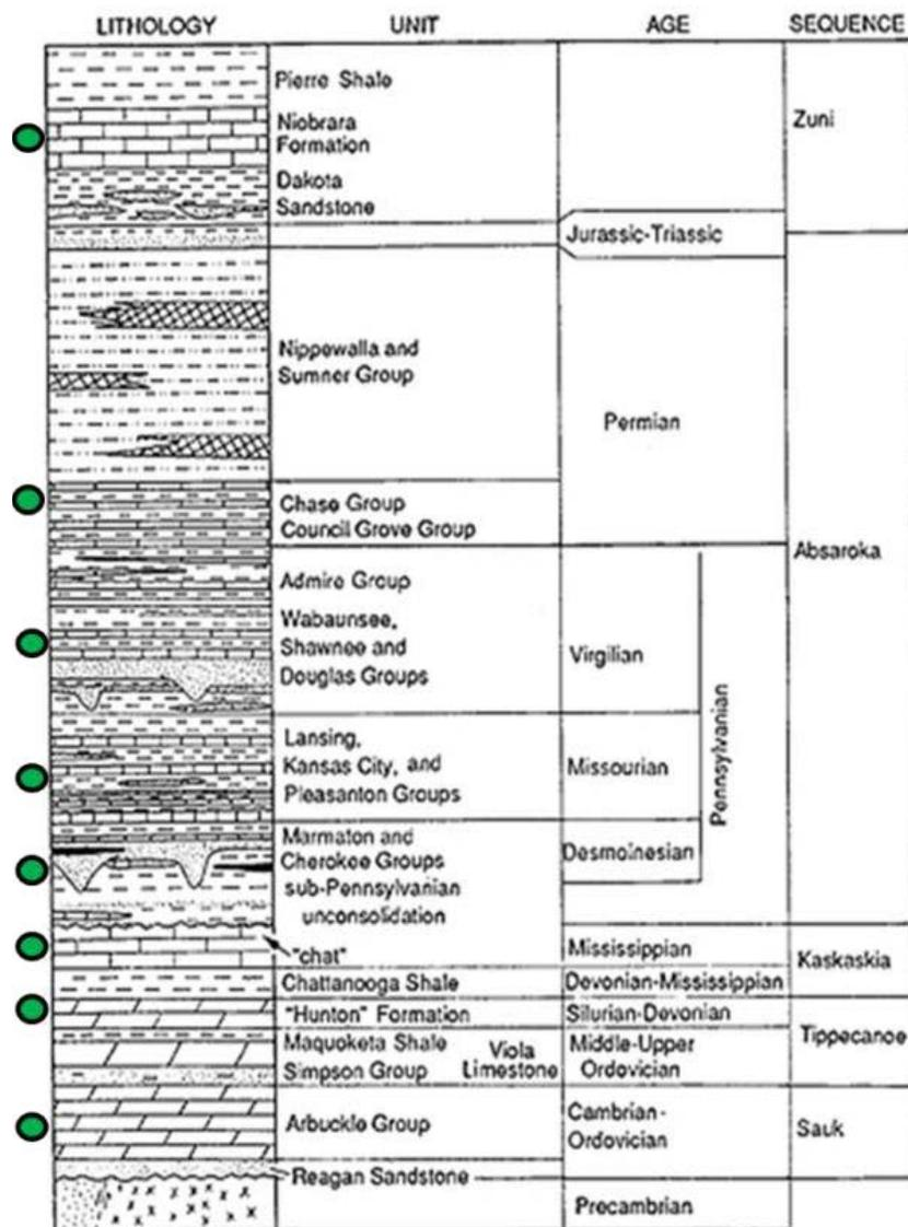
**Figure 4:** Kansas Stratigraphy and Petroleum Geology (Obtained from Moore et al., 1952 and modified). Green dots represent potential hydrocarbon-bearing units.
