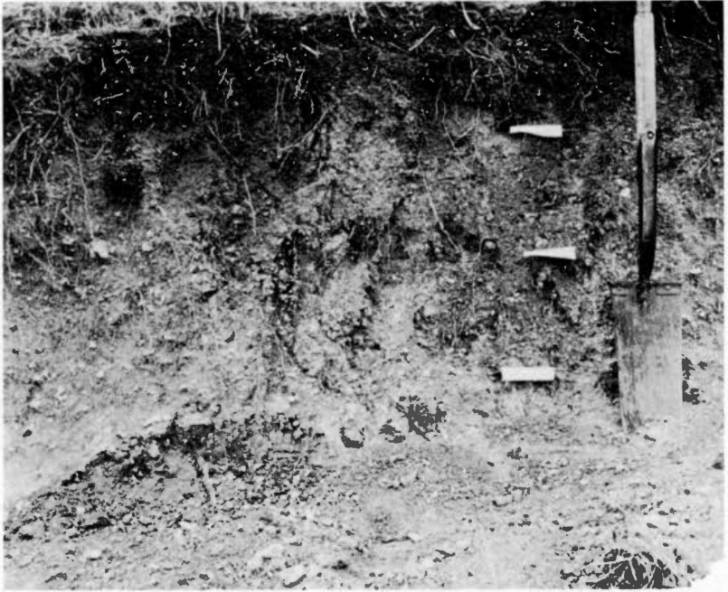
FIGURE 6. Soil profile of soil 3. The distance to the first marker represents the dark colored A1 horizon which is about 10 inches. The light colored spots in the lower portion of the profile are limestone fragments and lime concretions.
