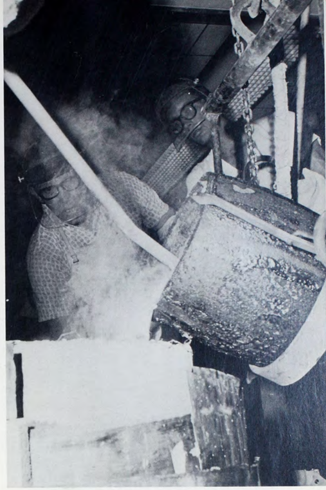
Molten metal emits intense heat as it is poured into a casting.
