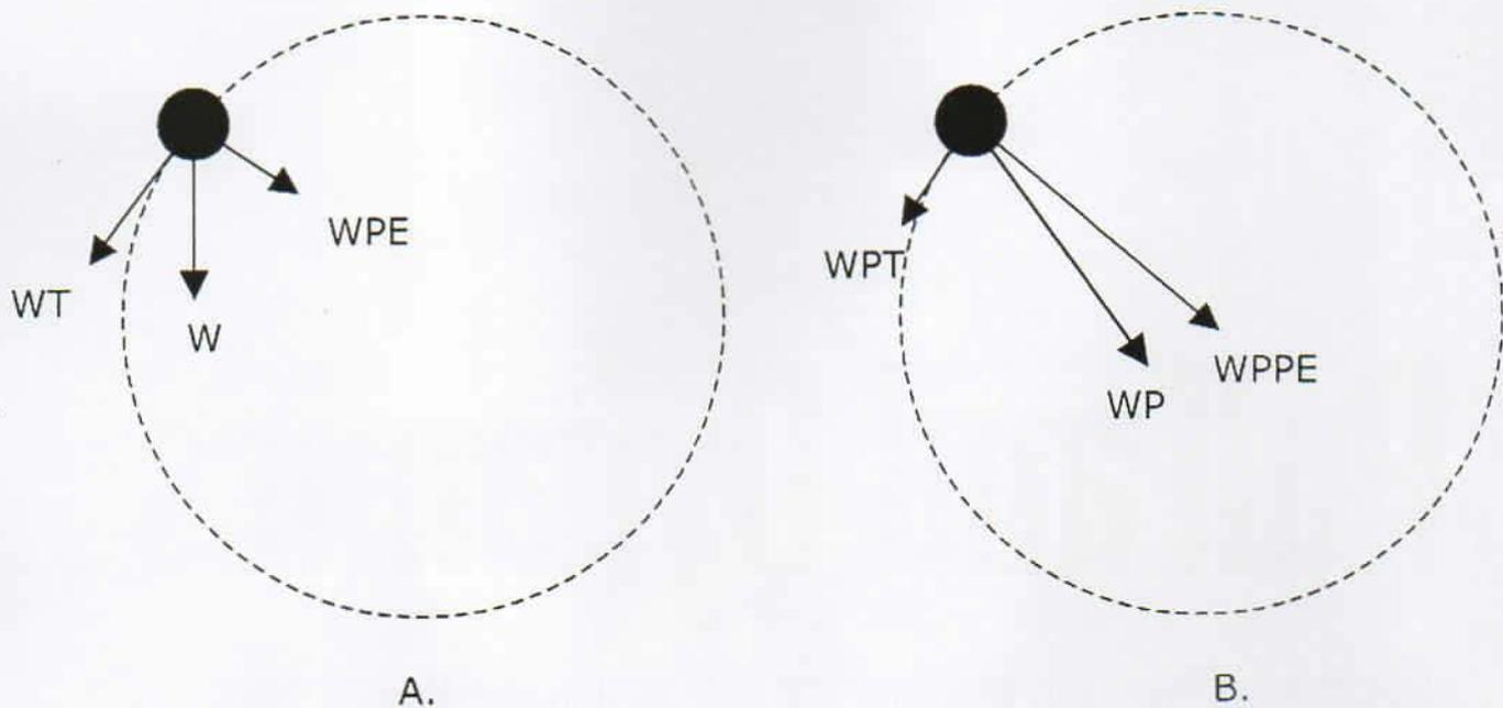
Figure 1. Forces acting on the hammer. A. Weight (W), tangential component of weight (WT), and perpendicular component of weight (WPE). B. Wire pull force (WP), tangential component of wire pull (WPT), and perpendicular component of wire pull (WPPE). The perpendicular components (WPE, WPPE) control the direction of motion of the hammer. The tangential components (WT, WPT) control the velocity of the hammer.
