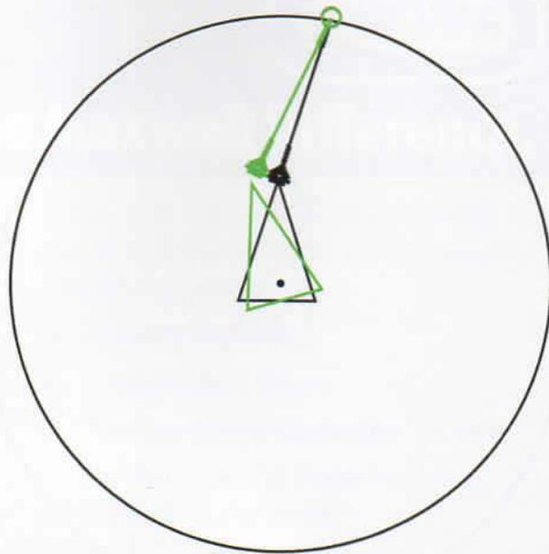
**Figure 4.** Pulling along the wire (green lines) where the latter points further ahead of the hammer's center of path
